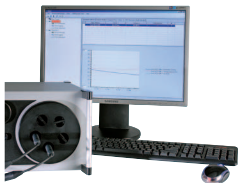
HygroGen2 chamber door with up to 6 probe connections. External monitor with HW4 software.
